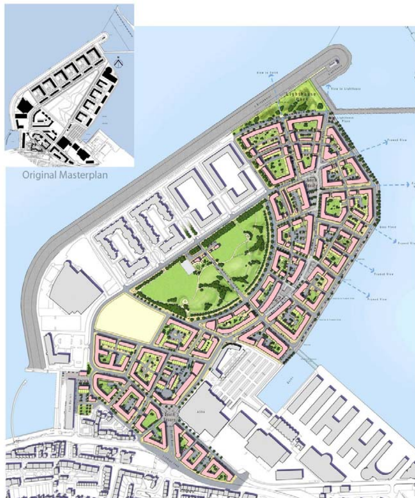
New Masterplan in colour with parts of the original Masterplan surviving due to completed sales shown in grey as other existing structures. The new Masterplan contains identical accommodation and open space provisions as the planned remainder of the original Masterplan.
