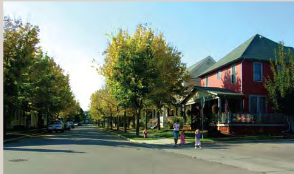
Residential streets like this 28-foot wide example in Prospect New Town in Longmont, Colo., are a staple of New Urbanism, but are often hindered by the International Fire Code's 20-foot clear rule. Properly designed, and in connected networks, these streets actually help emergency response times and calm traffic. (Photo courtesy of CNU)
