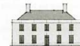
ii) Regular openings The openings on this 5 bay façade are equally spaced.
