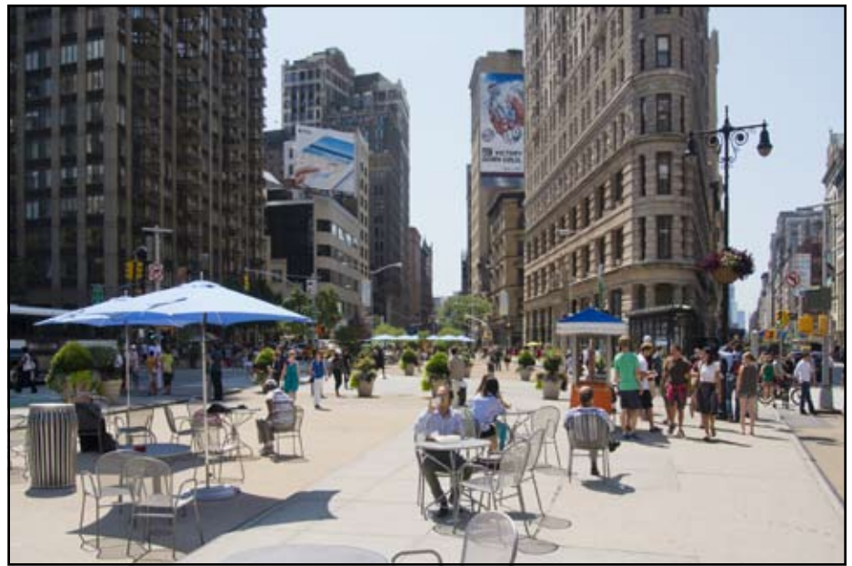
Madison Square, Broadway at 23rd Street, NY. “Tactical urbanism at its best,” Dover and Massengale say. New Yorkers immediately started enjoying the former expanse of asphalt after NYC DOT placed boulders to close large parts of the street to cars. Sections intended for seating were covered in a sand-colored, textured paint, and lightweight outdoor furniture was scattered around.
