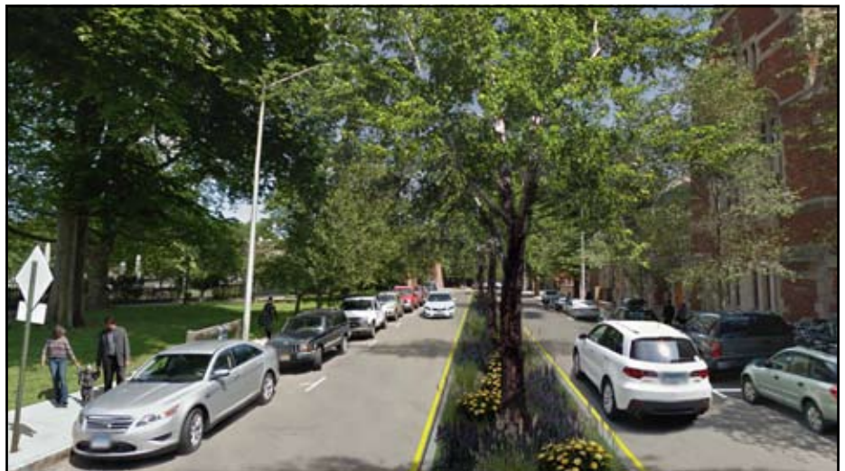
Existing Grove Street, top, is wide and fast-moving. The plan shows a median to narrow lanes. Below, the simpler plan for York Street allows a more immediate conversion with paint.
