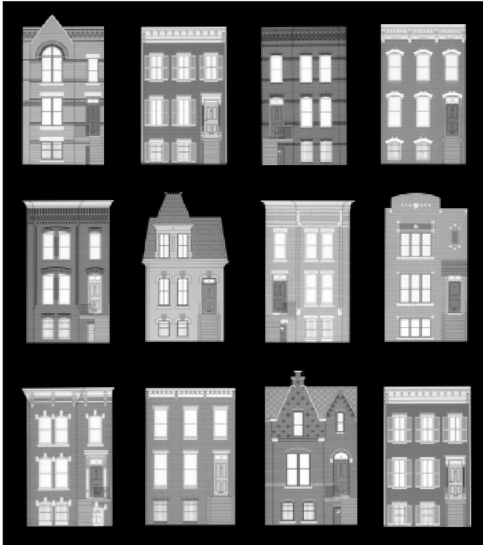
These are twelve of the twenty-three facade designs for Building Type 1, all of which have essentially the same floor plan.
