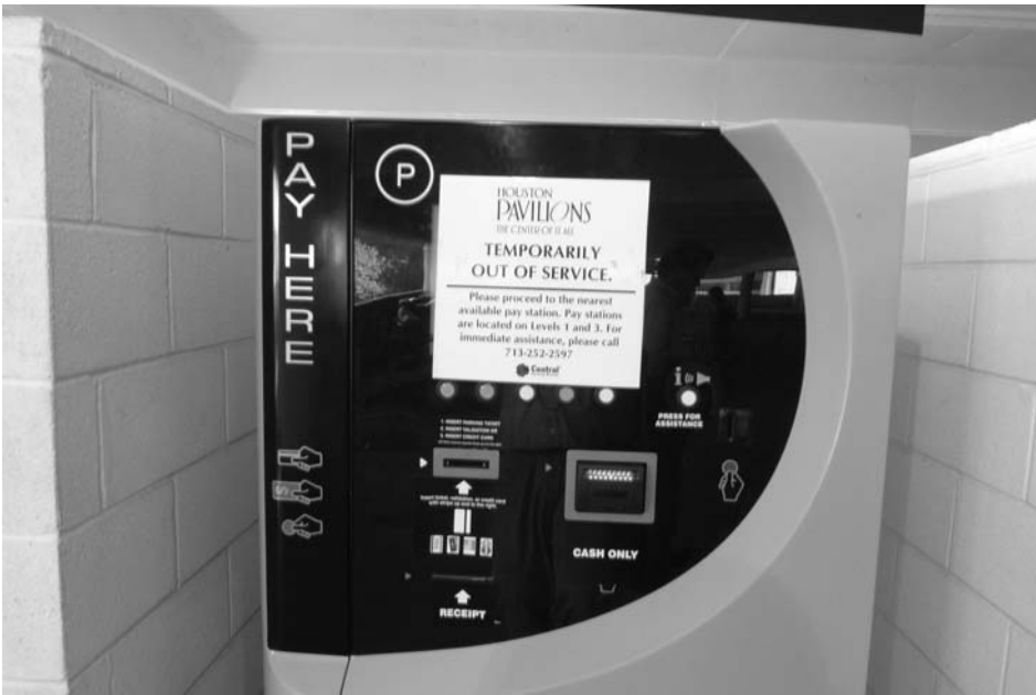
Figure 8-8 Parking machines often malfunction and should not be substituted for manned ticket booths in shopping center parking decks. Gibbs Planning Group, Inc.
