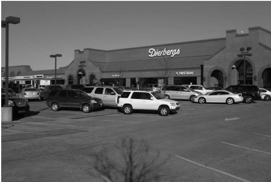
Figure 8-3 Most suburban and rural supermarkets require 250 or more parking stalls located adjacent to their front entry. Decked parking and smaller ratios can be supportable in dense urban locations. Robert J. Gibbs
